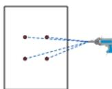
Drill the four marked holes using 5mm drill bit hand drill. The drilled hole depth should be 30mm.
