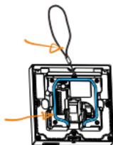
For the convenience of the installation, it is advised that you lead the rope we provided through the rope hole at the back of the device, then fill in the groove using the silicone foam strip.
