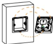
Make all cables go through the groove of the cable locking plate, then hang the device onto the junction box mounting bracket while pushing it down against the corresponding hook hanger.
