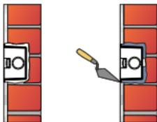
Cut out a square hole with the dimension (height\*width\*depth = 86\*86\*50mm). And lead a cable from the square hole in to the junction box .
