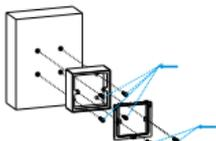
Fix the the junction box on to the wall using 4 ST4x20 screws, then fix the junction box component on to the junction box using 2 M4x30 screws.
