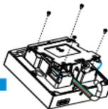
Insert the cable locking plate and tighten it using 4 M2.5x4 screws.
