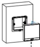
Push the device against the hook hanger and tighten the device with a M3x4 screw using Allen wrench as indicated in the drawing.
