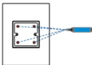
Mark the positions of the four holes of the Junction box at the hole center.
