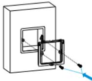
Fix the junction box component on to the junction box using 2 M4x30 Screws.
